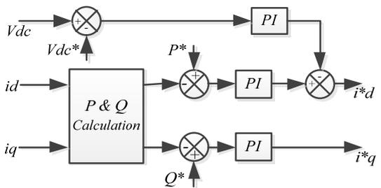
Fig. 5. Reference currents determination in grid-side converter controller.
