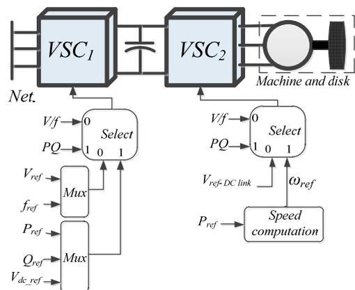
Fig. 8. The overall control structure of FESS.
