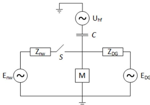
**Fig. 1** Structure of system impedance monitoring method [15].
