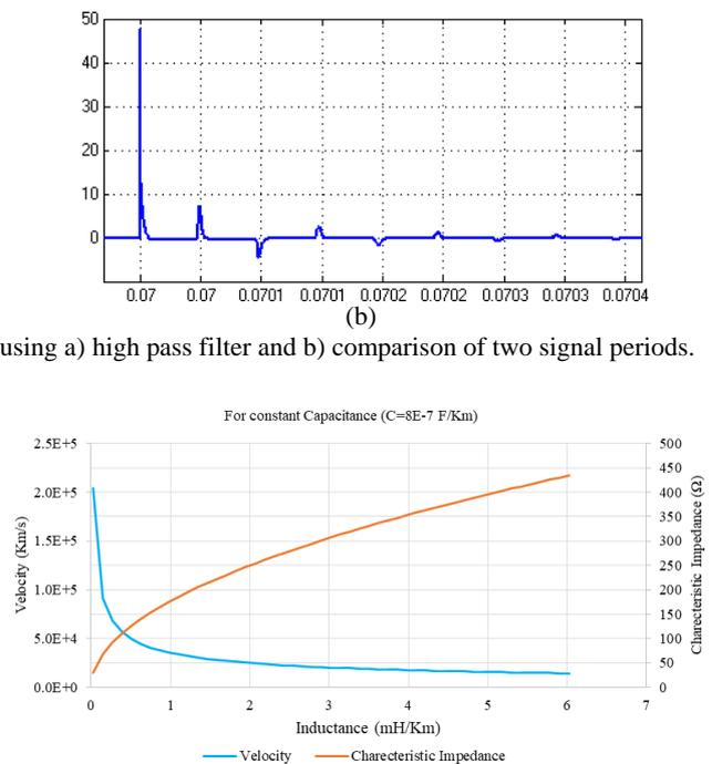
Fig. 14 Traveling speed and characteristic impedance curves for different inductance values.
