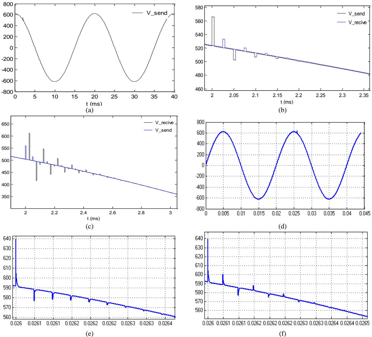
**Fig. 11** Simulation results in EMTP/rv a) system voltage wave form with injected pulse, b) traveling wave in receiver and transmitter side under normal conditions, c) traveling wave in receiver and transmitter side under islanding conditions-simulation results in MATLAB/Simulink, d) system voltage wave form with injected pulse, e) traveling wave in transmitter side conditions and f) traveling wave in transmitter side conditions.
