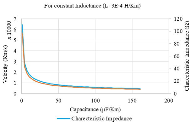
Fig. 13 Traveling speed and characteristic impedance curves for different capacitance values.
