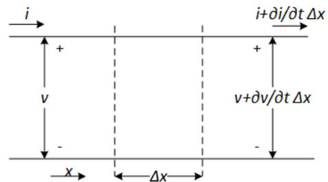
**Fig. 2** Part of distributed transmission line.
