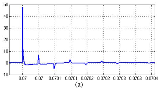
Fig. 12 Extracted traveling wave from system voltage wave form using a) high pass filter and b) comparison of two signal periods.
