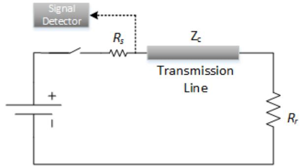
Fig. 4 Simple structure of proposed active method.
