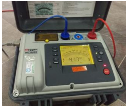
Fig. 10 Electric resistivity test of stress grading tubes.
