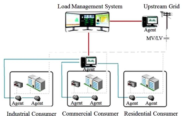
Fig. 1 Micro-grid structure based on agents.
