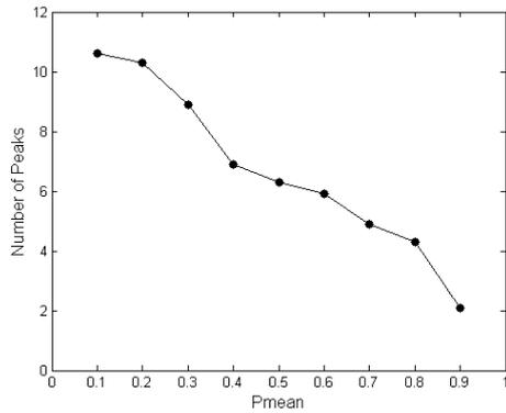
Fig. 3 The effect of the change in  $p_{mean}$  value on the mean of the number of peaks found in idPSO algorithm.
