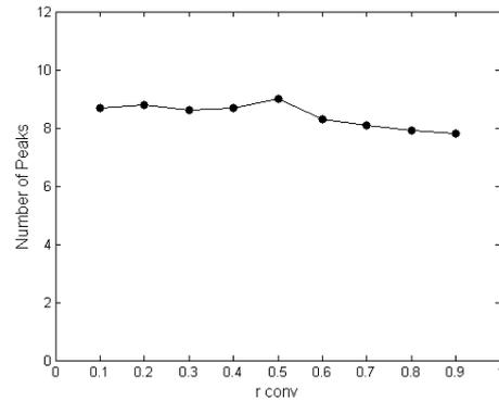
**Fig. 1** The effect of the change in  $r_{conv}$  value on the mean of the number of peaks found in idPSO algorithm.
