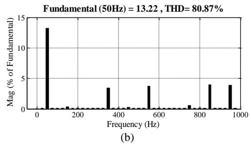
**Fig. 8** One phase output voltage and THD (PWM method).
