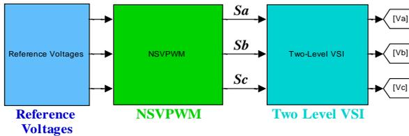
Fig. 3 Block diagram of the neural SVPWM a three-phase two level VSI.
