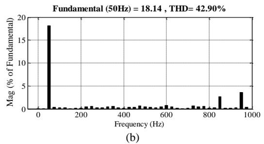
**Fig. 10** One phase output voltage and THD (neural SVPWM).
