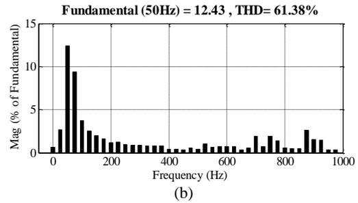
**Fig. 9** One phase output voltage and THD (SVPWM).
