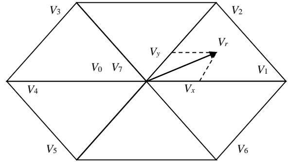
**Fig. 2** Principle drawing SVM for a three-phase two level VSI.
