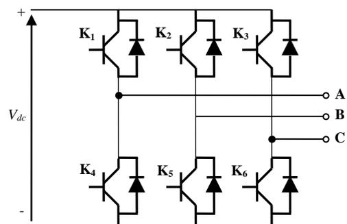
Fig. 1 Fundamental circuit of three phases two level VSI.
