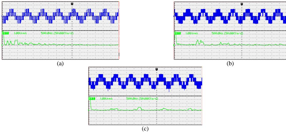
Fig. 12 Experimental results: output voltages and their spectra; a) PWM, b) SVPWM, and c) NSVPWM.
