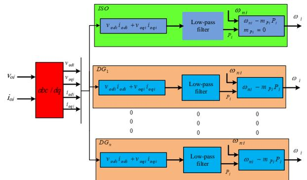
Fig. 2 Block diagram of active power controllers.
