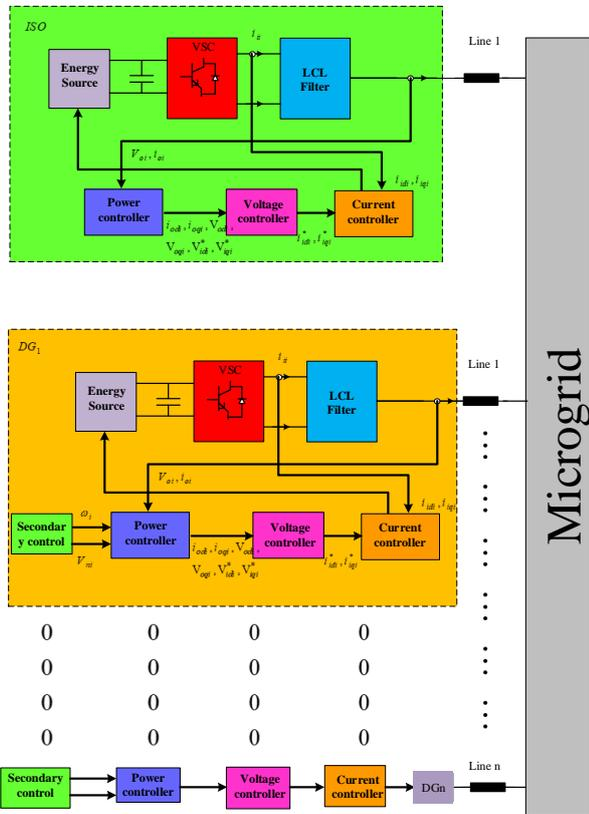
Fig. 1 Schematic diagram of a microgrid system.
