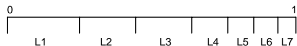
Fig. 2 The roulette wheel mechanism for the normalized probabilities of the load forecast levels
