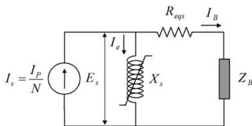
Fig. 10 Equivalent Simplified equivalent circuit of CT.
