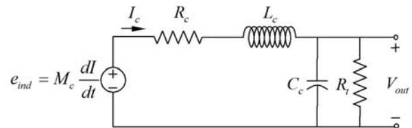
Fig. 2 Equivalent circuit of Rogowski coil.
