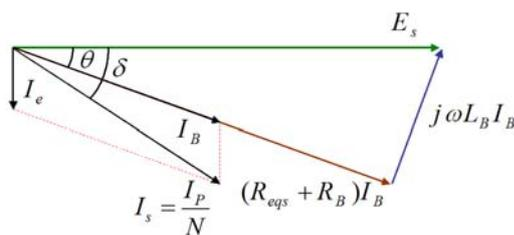
Fig. 11 Vector diagram of simplified equivalent circuit of CT.
