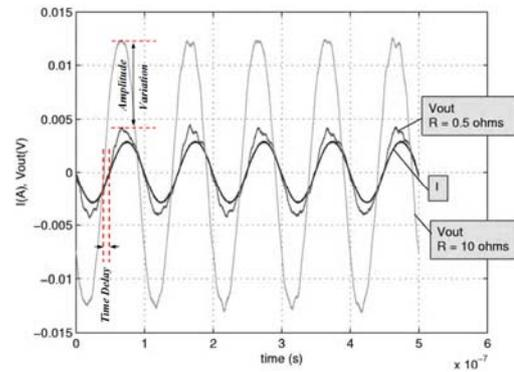
Fig. 8 Measured partial discharge using Rogowski coil [12].
