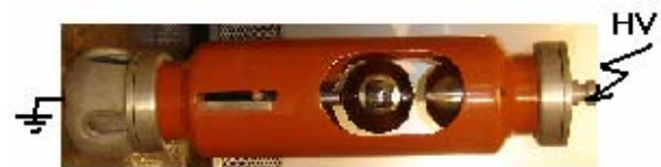
Fig. 2 Standard sphere-sphere electrode.
