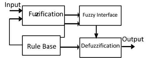
Fig. 6 Block diagram of the fuzzy logic system.
