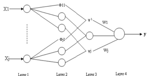
Fig. 4 Schematic of Wavelet Network.
