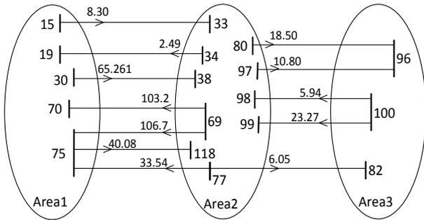
Fig. 4 Magnitude of power flow (MW) in tie-lines.
