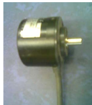
Fig. 2 The ten bit absolute encoder.
