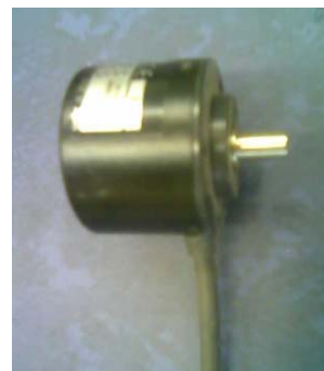
Fig. 2 The ten bit absolute encoder.
