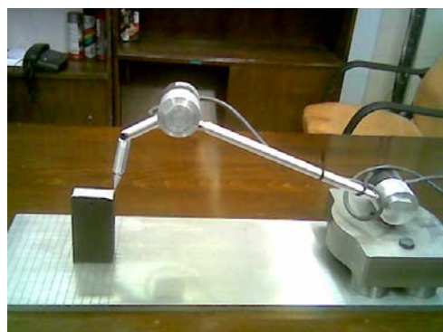
Fig. 1 The three degree of freedom manipulator.
