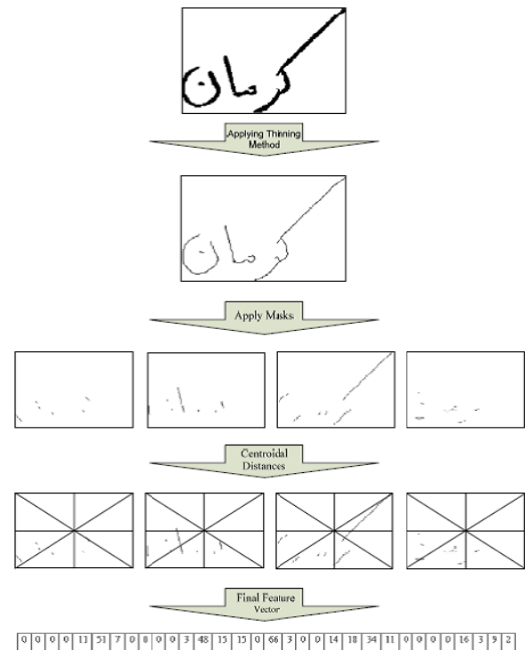
Fig. 2 The stages of the applied feature extraction method for Persian handwritten word recognition.
