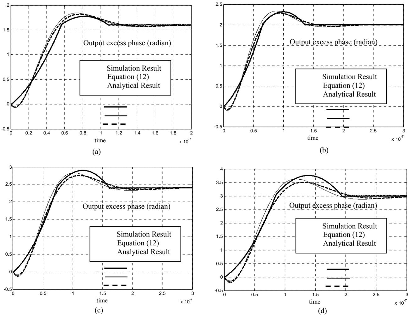
**Fig. 5** Comparison between approximated and numerical results of Eq. (12) and simulation results for output excess phase when input phase step increases. (a)  $\Delta\phi_{in} = 0.8\text{rad}$  , (b)  $\Delta\phi_{in} = 1\text{rad}$  , (c)  $\Delta\phi_{in} = 1.2\text{rad}$  , (d)  $\Delta\phi_{in} = 1.5\text{rad}$ .
