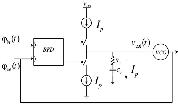
**Fig. 1** BBPLL architecture with first order filter
