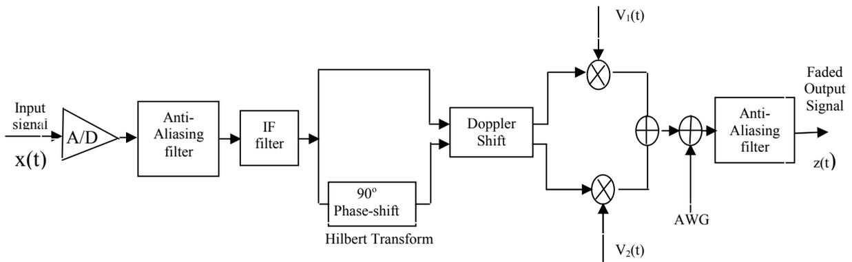
**Fig. 4** One diffused component(with Doppler) hardware simulator.
