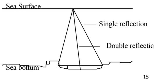
**Fig. 2a** Single and multiple specular reflections
