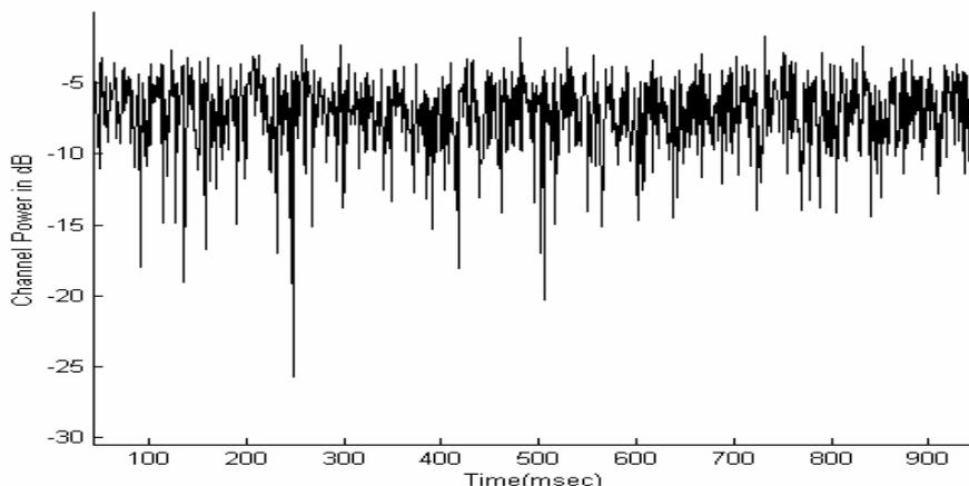
Fig. 9 Shallow water base-band channel amplitude fluctuation
