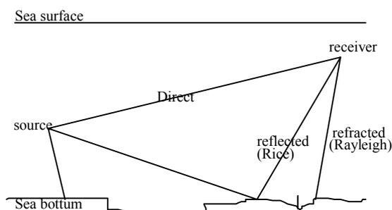
**Fig. 2b** Source and receiver paths picture
