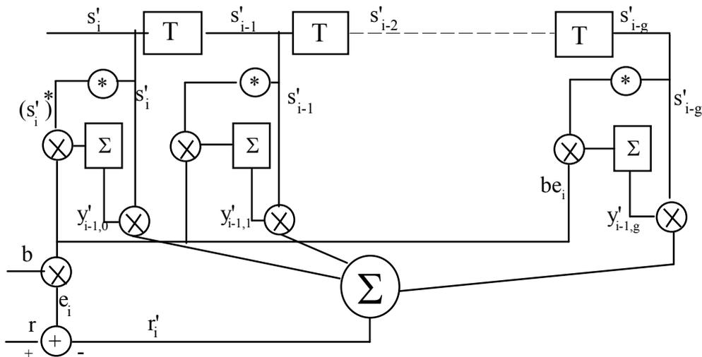
**Fig. 7** Complex linear feed-forward estimator with degree zero prediction
