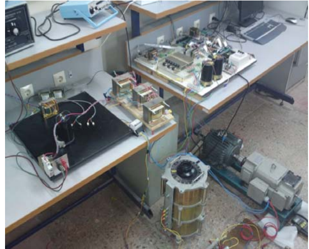
Fig. 4 SRM drive test setup used for experimentation.
