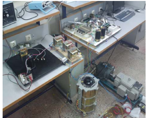
Fig. 4 SRM drive test setup used for experimentation.
