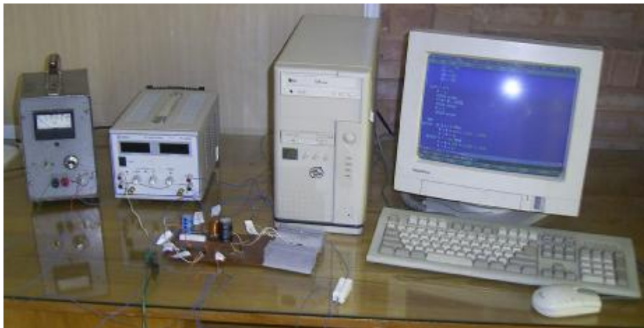
Fig. 9 The constructed fuzzy MPPT system.
