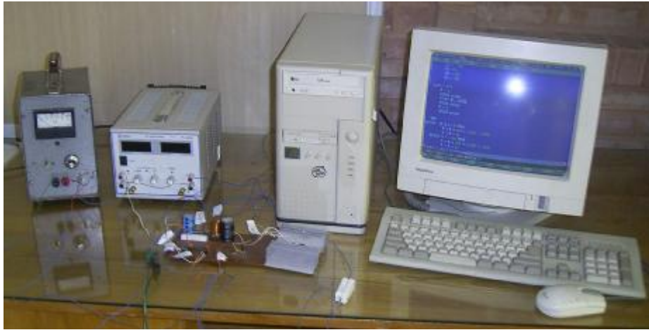
Fig. 9 The constructed fuzzy MPPT system.
