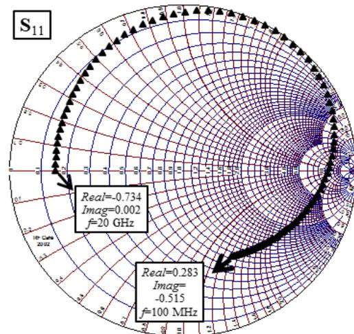
Fig. 12 S-parameter of the AI for medium frequencies.
