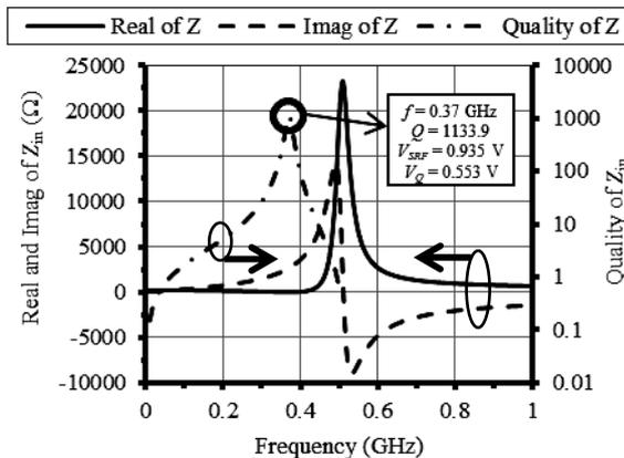
**Fig. 6**  $Z_{in}$  and its QF in low frequencies.
