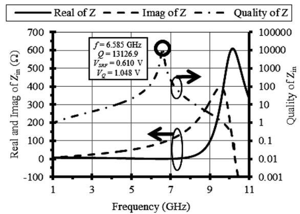
**Fig. 7**  $Z_{in}$  and its QF in medium frequencies.
