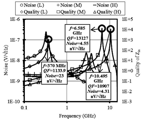
**Fig. 10** Noise and QF of the AI.
