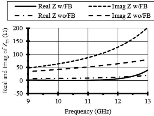
**Fig. 5** Input impedance  $Z_{in}$  in high frequencies, with and without local feedback.
