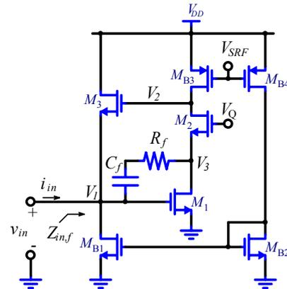
**Fig. 2** Schematic of the proposed AI circuit.
