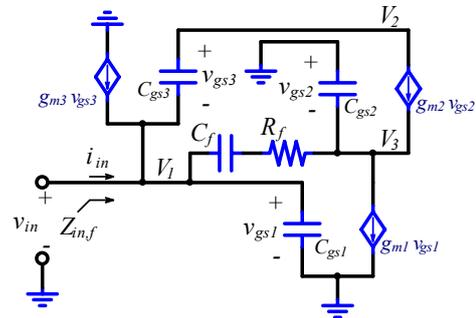
**Fig. 3** Small-signal equivalent circuit of the proposed AI.
