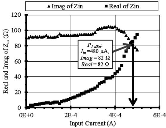
Fig. 13 Linearity of the AI at 6.585 GHz.
