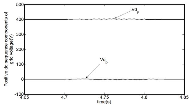
Fig.27 Positive dq sequence components of grid voltage
