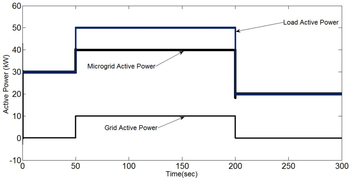
Fig.9 Active load, microgrid and grid power
