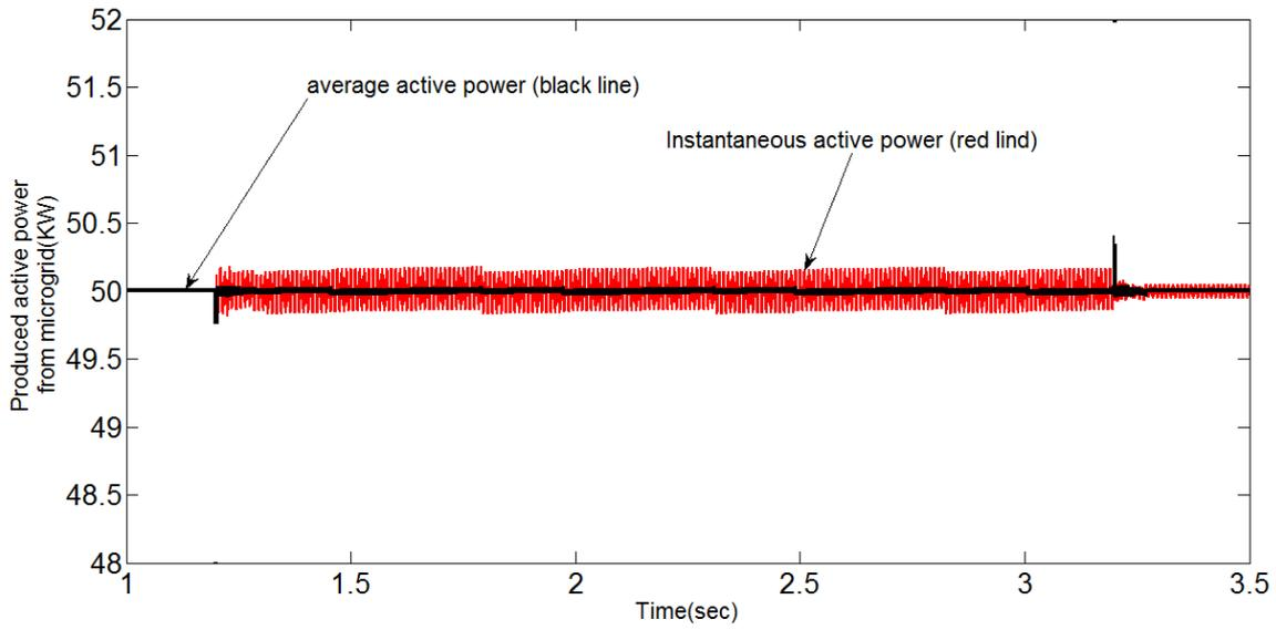
Fig.17 average and instantaneous active power of microgrid
