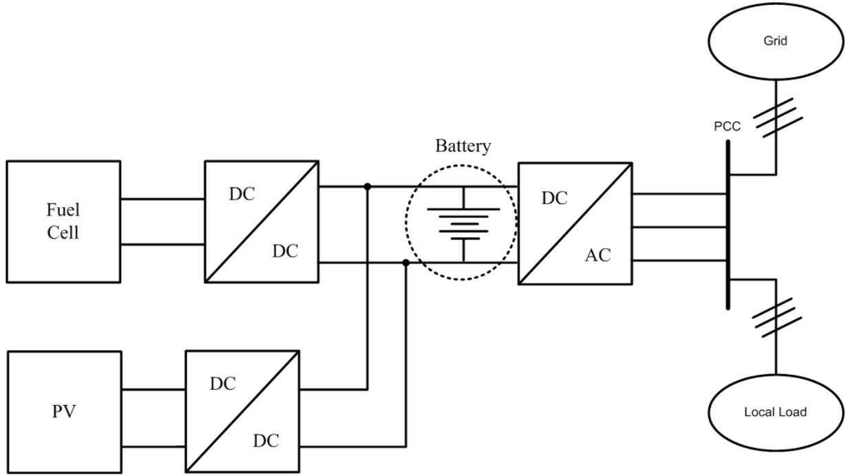
Fig 1: Hybrid Renewable energy sources in a microgrid
