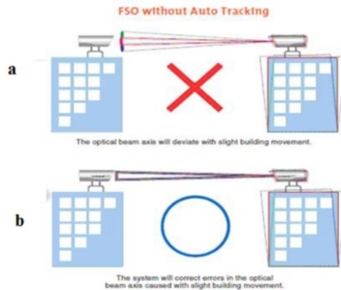
Fig. 5: Schematic representation of the auto-tracking subsystem effect, canon company.
