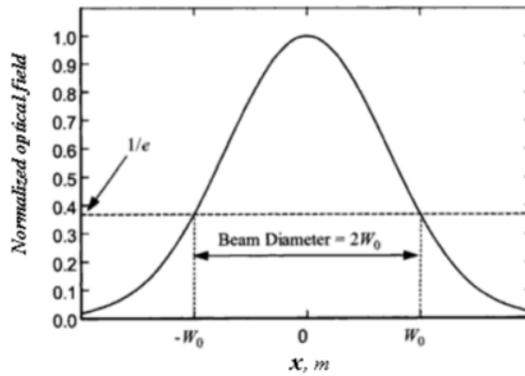
Fig. 3: Amplitude profile of a Gaussian beam wave [9].
