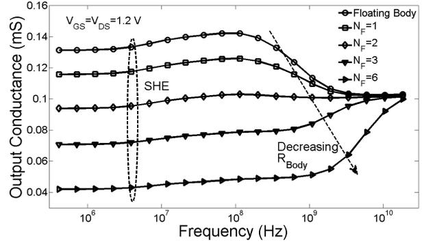
**Fig. 4** Output Conductance vs. Frequency at  $V_{GS}=V_{DS}=1.2$  V.
