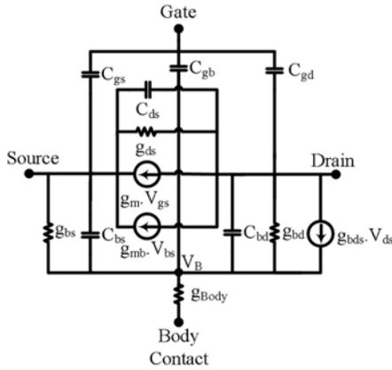
Fig. 6 Small-signal model of PD SOI MOSFET.
