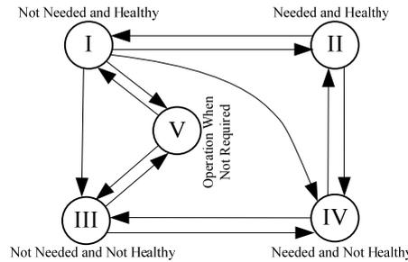
Fig. 2. Reliability model for protection systems [6].
