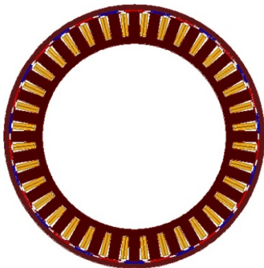
Fig. 1 Permanent-magnet outer-rotor synchronous generator.
