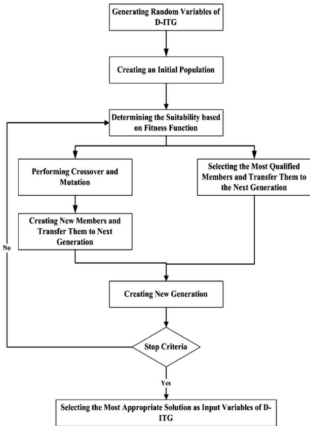
Fig. 2 Flowchart of GA based proposed algorithm.
