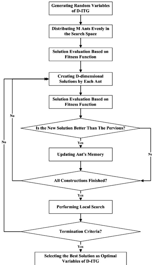
Fig. 4 Flowchart of ACO based proposed algorithm.
