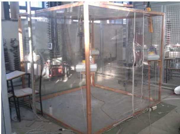
Fig. 3 Fog chamber for experimental tests.
