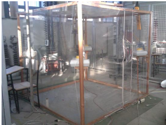
Fig. 3 Fog chamber for experimental tests
