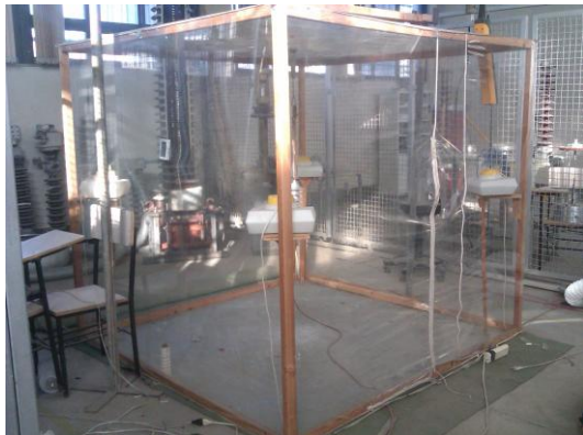
Fig. 3 Fog chamber for experimental tests
