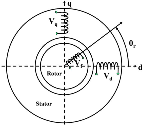
Fig. 1 Resolver model [12].
