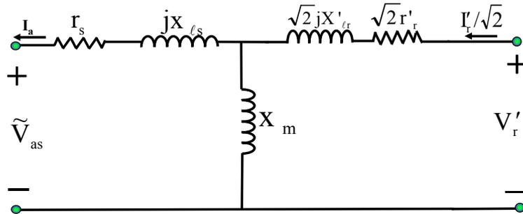
Fig. 3 Steady state equivalent circuits of the resolver.
