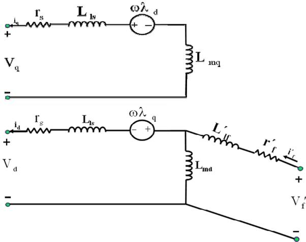
**Fig. 2** Dynamic electrical equivalent circuits of the resolver.
