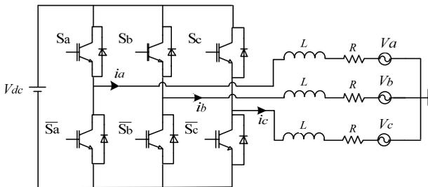
Fig. 1 Grid-connected three-phase VSC.
