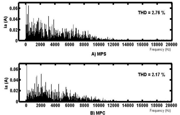
**Fig. 5** Harmonic spectrum of MPS and MPC.
