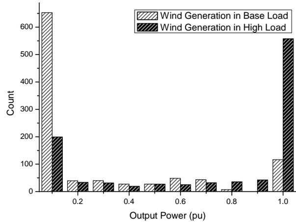
Fig. 5 Output Power for an instance Wind Turbine.
