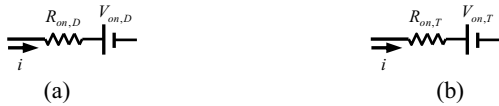
Fig. 7 (a) Turned on model of a diode; (b) Turned on model of a transistor.
