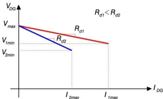
Fig. 2. A conventional droop control for two DGs
