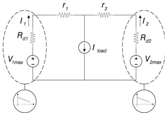
Fig. 1. A simple DC microgrid with two DGs
