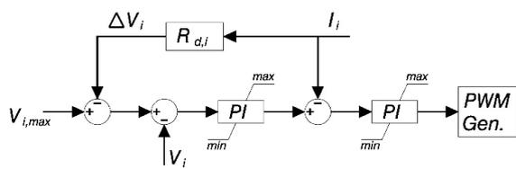
Fig. 8. Control block of the proposed droop scheme.
