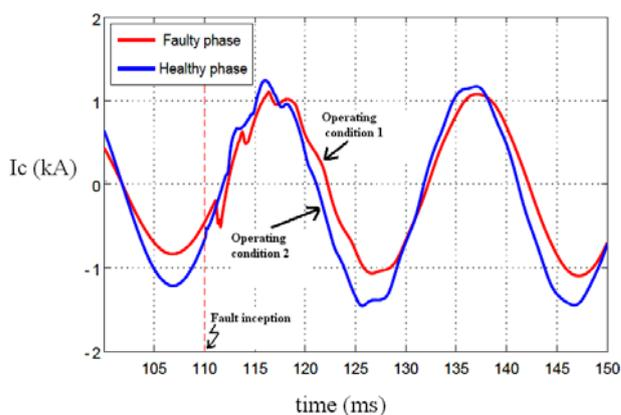
**Fig. 1** Phase current at two different operating conditions. Operating condition 1:  $\delta = 20^\circ$ ,  $L_f = 0.95^{p.u.}$ ,  $R_f = 200 \Omega$ . Operating condition 2:  $\delta = 30^\circ$ ,  $L_f = 0.05^{p.u.}$ ,  $R_f = 0 \Omega$ .
