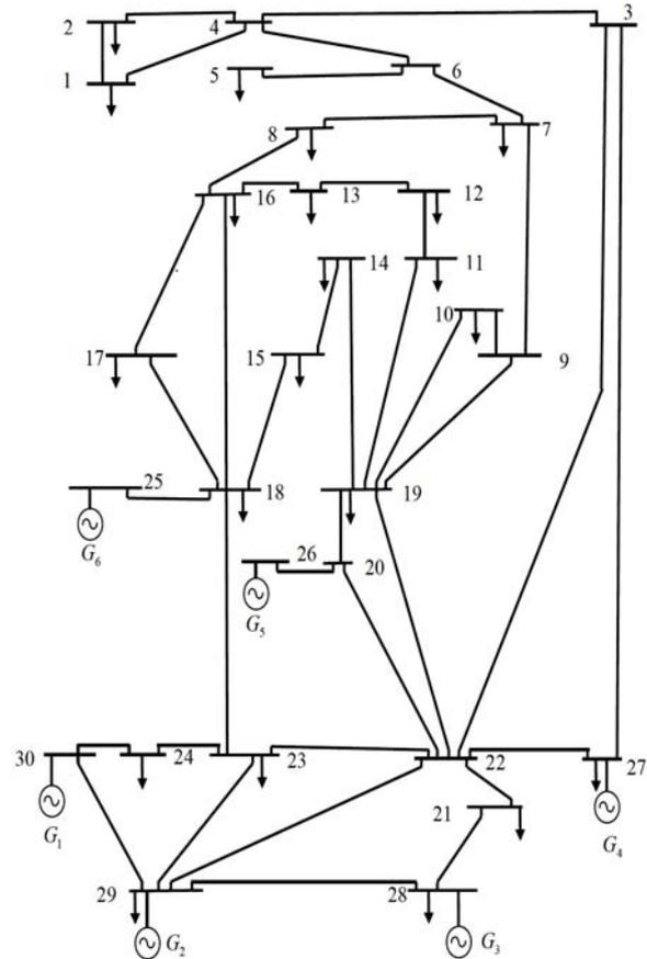
**Fig. 2** Single-line diagram of IEEE 30 bus test system
