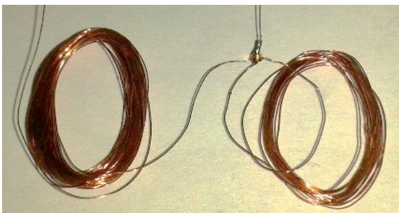
Fig. 7 The practical representation of short circuit in coils.
