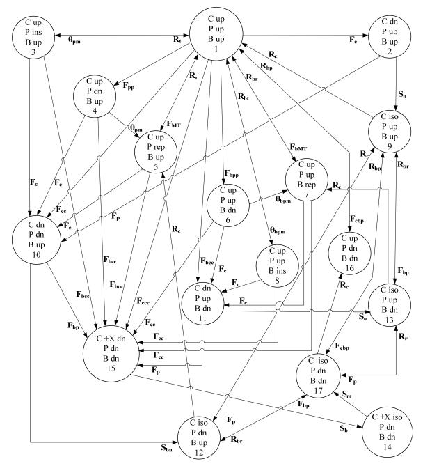
Fig. 1. Proposed extended Markov model of protected component and protection systems
