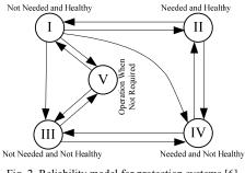
Fig. 2. Reliability model for protection systems [6].
