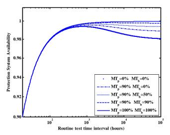
Fig. 4. Protection system availability with respect RTTI for different values of monitoring test effectiveness
