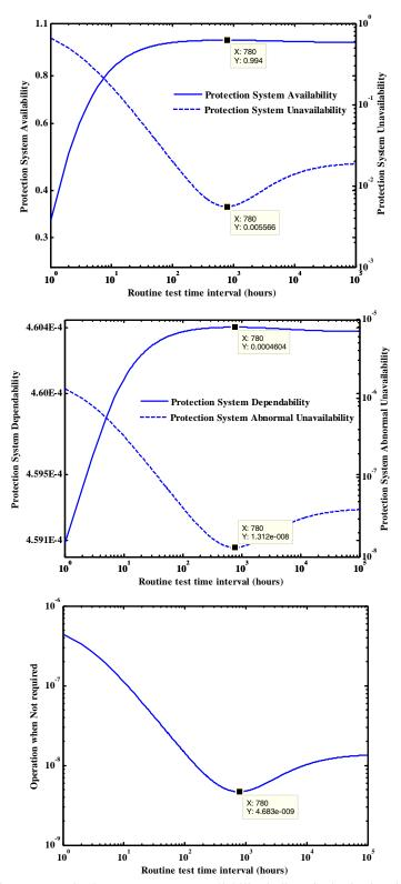
Fig. 3. Protection/component system reliability indices for basic situation
