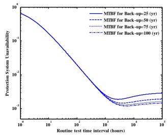
Fig. 5. Protection system unavailability with respect to RTTI for different values of MTBF<sub>b</sub>
