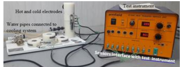
Fig. 9 Test set up to obtain thermal conductivity.
