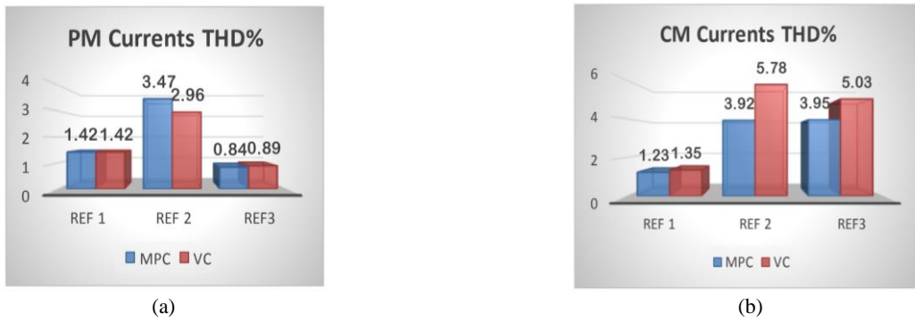
Fig. 7 THD values of the steady-state: a) PM and b) CM stator currents for VC and proposed methods.
