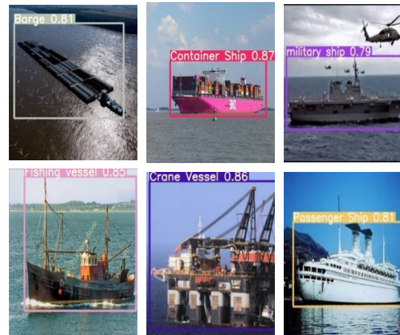
Fig. 15 The result of the custom model test dataset for ship detection using the Yolov5 network architecture.
