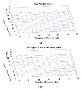
**Fig. 13** The combinations of the mover/stator number of coils on sensor's accuracy: (a) MPE, and (b)AAPE
