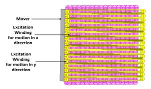
Fig. 1 The Mover ferromagnetic core and excitation windings
