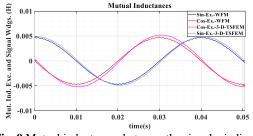
Fig. 9 Mutual inductances between the signal windings with the excitation winding
