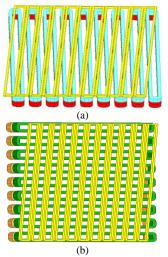
**Fig. 18** Using a skewed excitation winding for planar resolver (the back-iron is removed to clearly show the windings: (a) skewed excitation winding and the non-skewed x-signal windings, and (b) skewed excitation winding and the non-skewed y-signal windings
