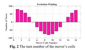
calculated based on windings' turn function. Since there is no slot-tooth region and the flux density in the back iron is in the linear part of the magnetization curve of the core material, the performance of the studied resolver is only influenced by the windings' distribution. On the other hand, the winding function method precisely consider the windings configuration. Therefore, is can be
