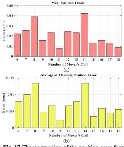
**Fig. 17** The worst value of the position error for the given number of mover coils: (a) MPE, and (b) AAPE
