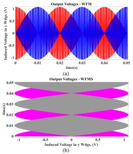
**Fig. 10** The induced voltages in the signal windings of planar resolver, calculated by winding function model: (a) x-direction windings, and b) y-direction windings.
