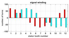
Fig. 4 The number of turns on each stator's tooth, red: cosine coils, and turquoise: sine coils
