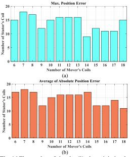
Fig. 16 The number of signal coil's that minimize the position error for a specific number of mover coils: (a) MPE, and (b) AAPE
