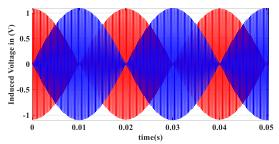
Fig. 19 The output voltage of x-signal windings using the skewed excitation winding.
