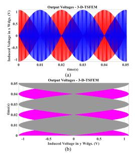
**Fig. 11** The induced voltages in the signal windings of planar resolver, calculated by 3-D TSFEA: (a) x-direction windings, and b) y-direction windings.
