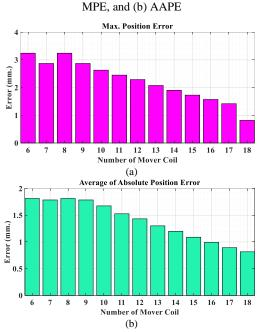
**Fig. 15** The worst value of the position error for the given number of mover coils: (a) MPE, and (b) AAPE
