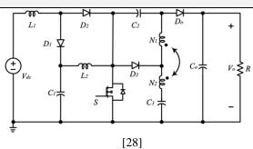
In a traditional SEPIC (single ended primary-inductor converter) design, a linked dual winding transformer with a turn ratio of n = (N1/N2) takes the place of the intermediate inductor.
