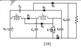
Three duty cycle models were proposed (0.0-0.7), and model III's 16 components allowed for a maximum voltage gain of 45.
