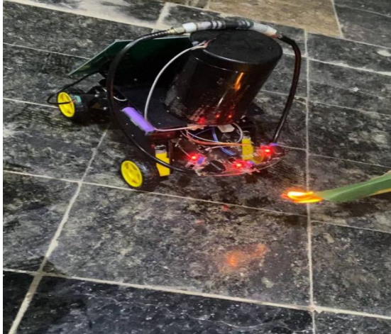
Fig.(16) Fire Fighting robot implementation.
