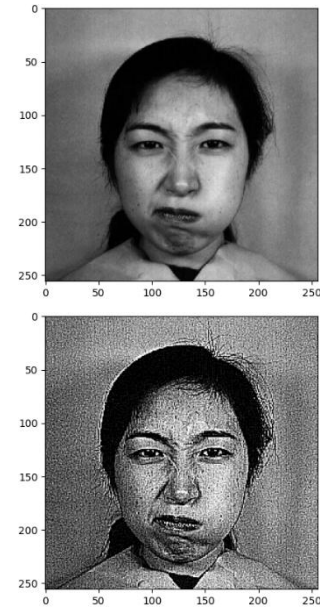
Fig. 8 Butterworth highpass filter
