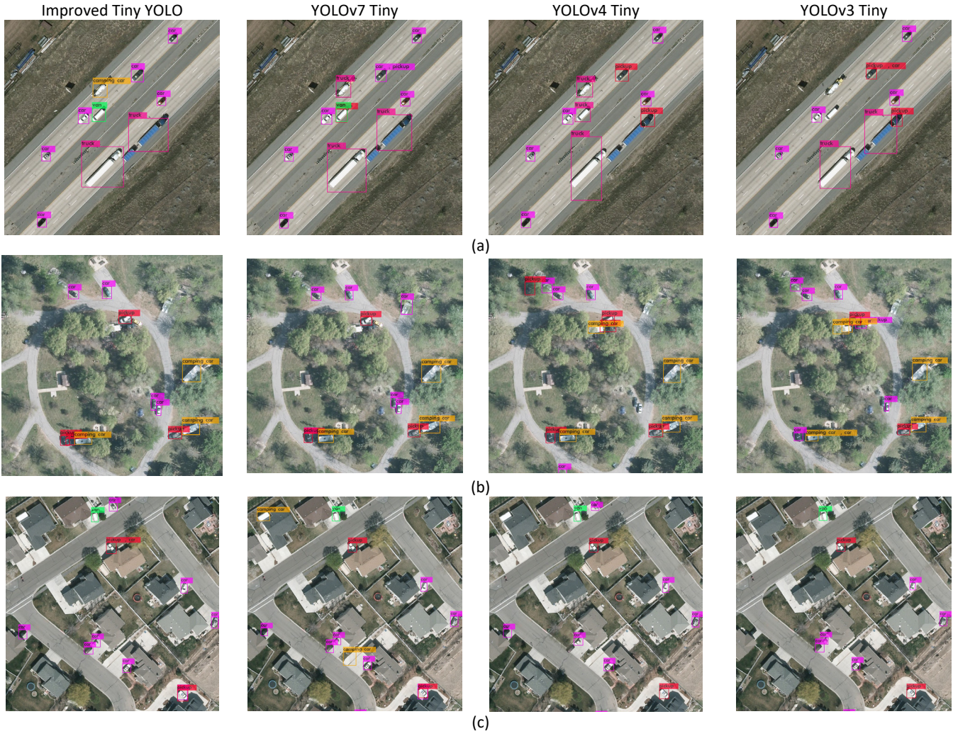
Fig. 5 Comparison of visual detection on test images. (a) Varying sizes (b) Occlusion (c) Complex background.
