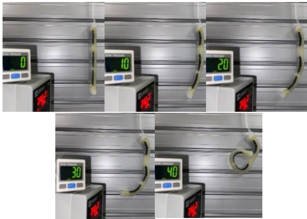
Fig 13. Segmented bending actuator motion in response to every 10 kPa incremental input pressure.
