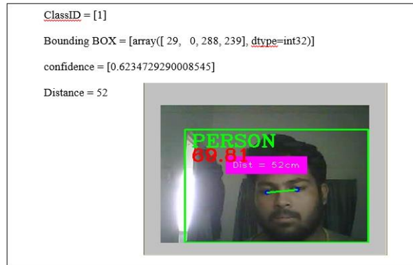
Fig. 8a Image display of face in real-time along with confidence value
