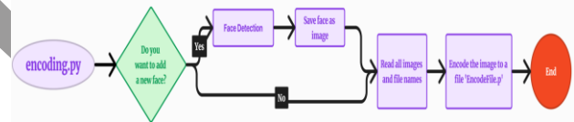
Fig. 2 working procedure for addition of new faces
