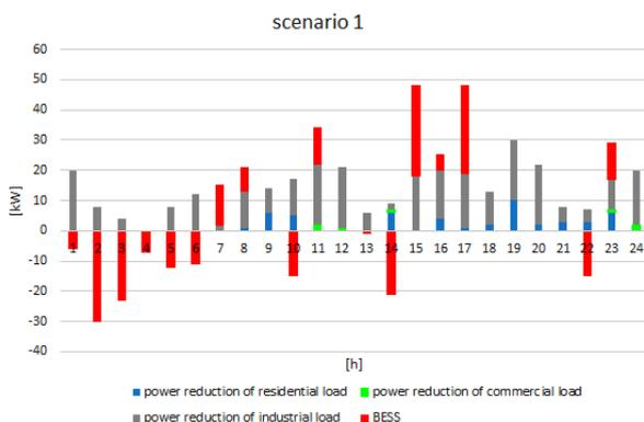
**Fig. 6** Power of BESS and power of the consumers in scenario 1.
