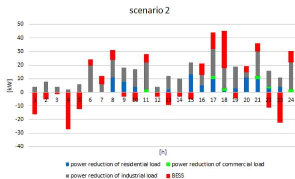
**Fig. 7** Power of BESS and power of the consumers in scenario 2.
