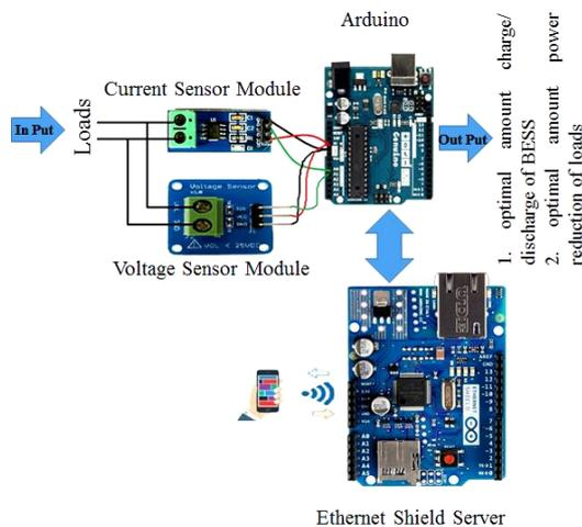
Fig. 3 The proposed implementation of the load management system for each of the consumers.
