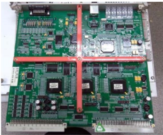
Fig. 7 The motor control single board case of in DCU control motor.
