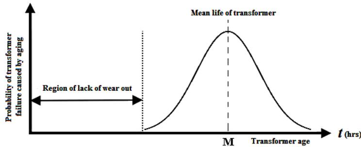
Fig. 3 The failure distribution function of the transformer considering wear out period.
