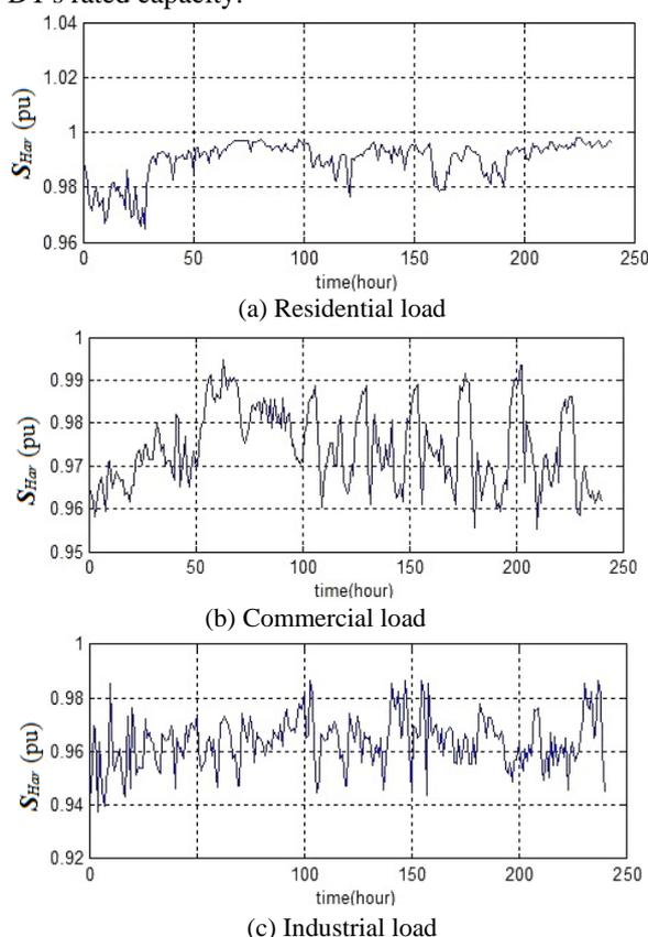
**Fig. 5** The available capacity of DT associated with the first 10 days of measurement in the presence of the harmonic ( $S_{Har}$ ) for three kinds of loads.
