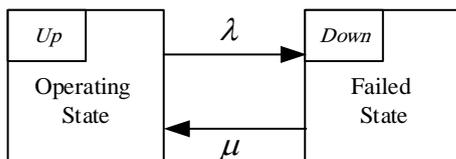
Fig.1 State space diagram of a repairable component.
