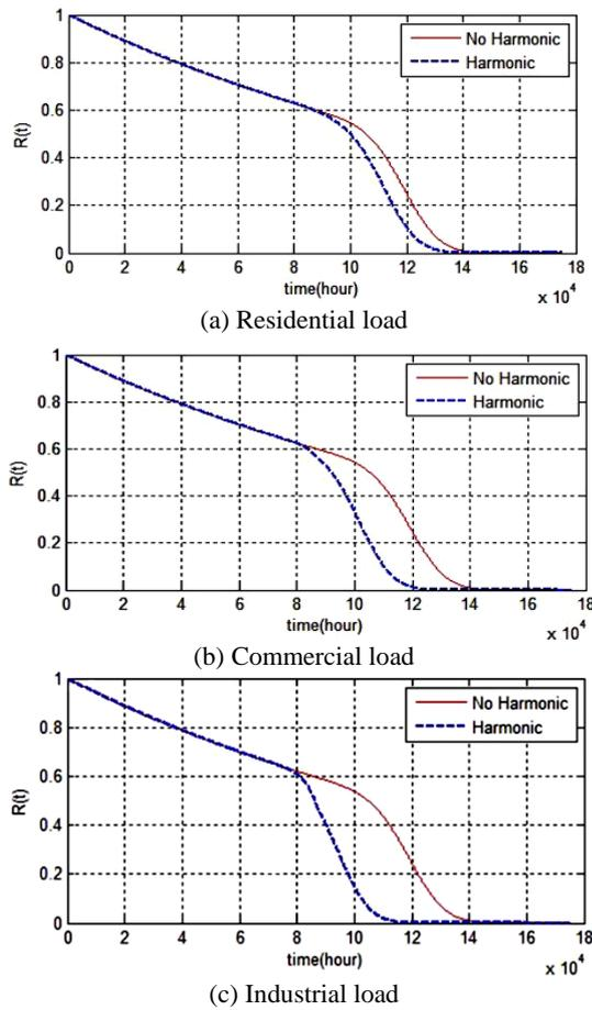
**Fig.6** The comparative diagram of the DTs' overall reliability with and without considering the harmonic.
