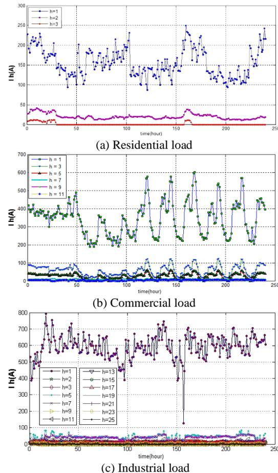
Fig. 4 Diagrams of the DT's harmonic amplitude associated three kinds of loads.
