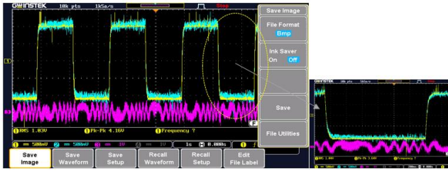
Fig. 10 The dynamometer torque response for the pulse torque reference T_0=\pm 3 N.m
